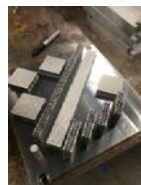
Ti6V4Al Lattice Structure Metal Prints EOS M290
